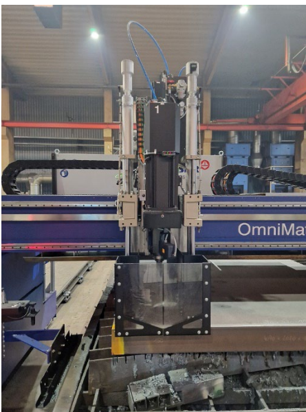
Image 2: The drilling unit now enables effortless pre-drilling of start holes and cutting the smallest contours into thick material. © Messer Cutting Systems
