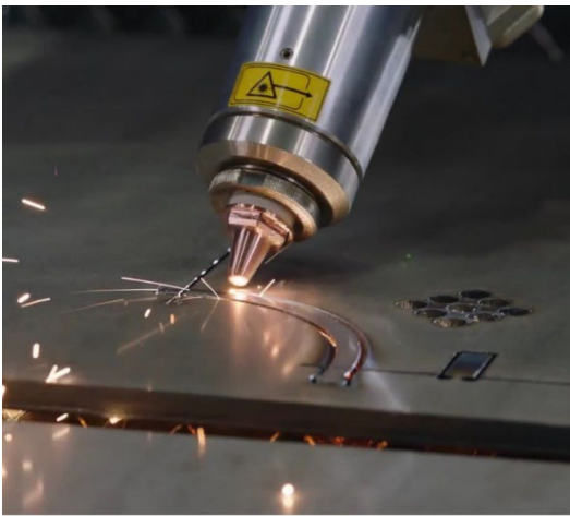
Pic 1: The Bevel-U bevel unit of the ELEMENT L laser cutting system delivers a wide variety of bevel contours in the best and standard-compliant cutting quality, even with material thicknesses of 50 mm. © Messer Cutting Systems
