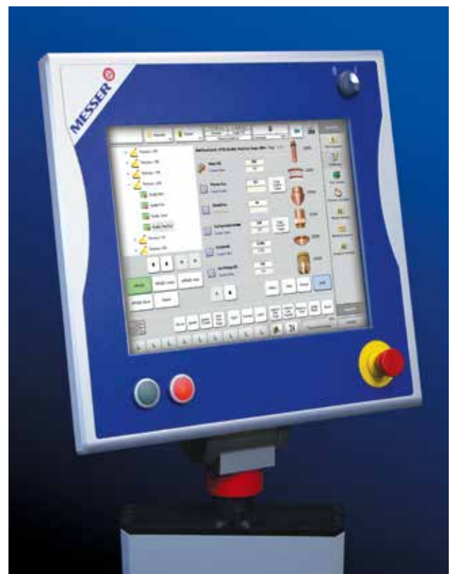
High strength machined aluminium enclosure
