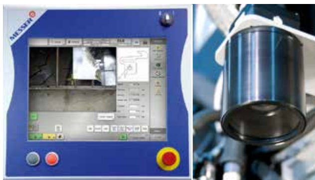
Video camera featured above (right) allows for fast, accurate plate alignment.
