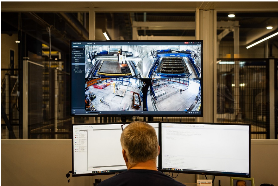
Photo 4: Production is automated to the greatest possible extent and exclusively controlled from a control room. © Messer Cutting Systems
