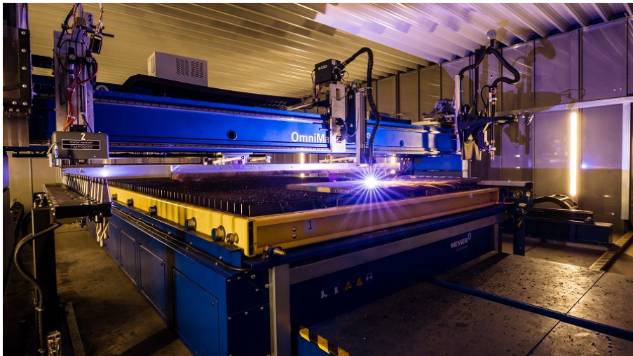
Photo 6: OmniMat® cutting machine equipped with the Skew Delta plasma bevel unit for weld preparation © Messer Cutting Systems
